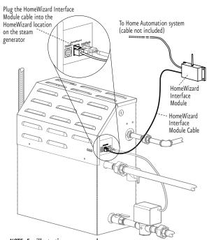
NOTE: For illustrative purposes only. The eTempo control cable is not shown for clarity. An eTempo or eTempo/Plus must be used in conjunction with the HomeWizard.
