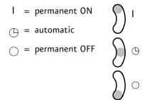
**IMPORTANT:** It is recommended that for periodic and effective blowdown, the override switch be set in the ( automatic setting.
