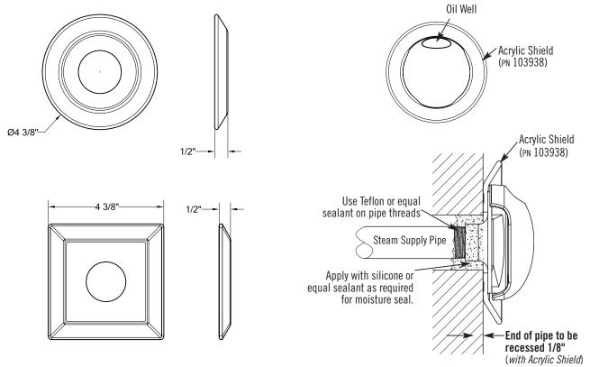
The Acrylic Shield (PN 103938) is for use when acrylic or other non-heat resistant materials are used for the steamroom enclosure.
